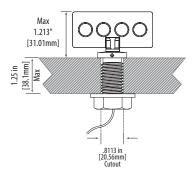
Bushing Mount provides the finished look of a ferrule at fixture base, allows 360° rotation of fixture head; position can be fixed with set screw. Bushing is attached with nut on rear side of mounting surface. Maximum mounting surface thickness 1.25" [38.1mm].
