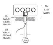
Stem Mount provides most minimal mounting option; stem attaches with nut on rear side of mounting surface; no rotation. Choose ST1 or ST2 based on the thickness of mounting surface.
