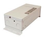
Load: 100W Total Input Voltage: 120-277 V 50/60Hz Output Voltage: Four Channel 24 V each Dimensions: 9.70"L x 4.07"W x 2.93" H
